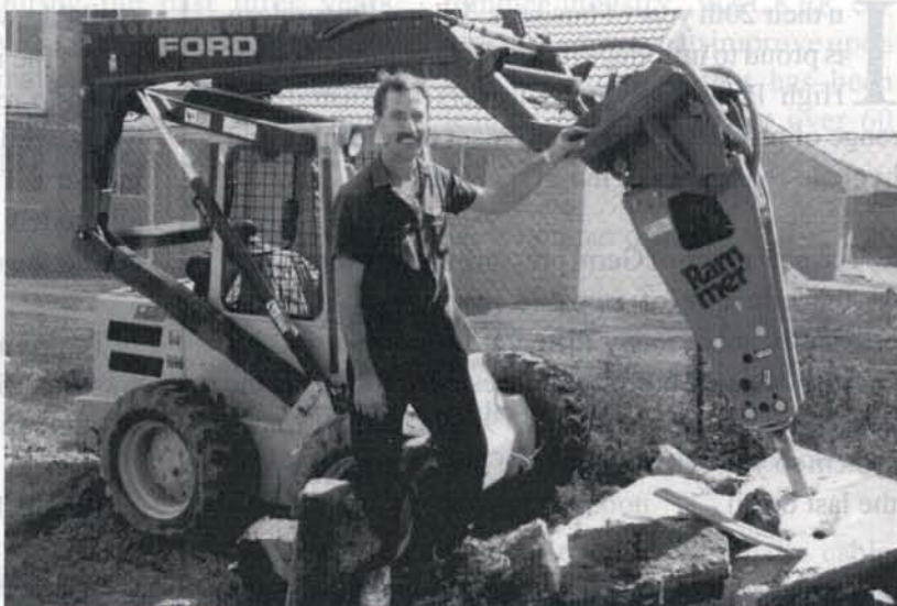
Con Vatos of C&G Earthmoving, said that the Rammer S23 hydraulic hammer, attached to his Ford L555 skid steer loader is proving a highly flexible and efficient equipment combination.
